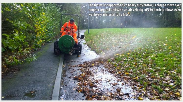
• The LBV Blower can be supplied with a variety of mounting frames and PTO speeds to suit tractor front or rear linkage or special
