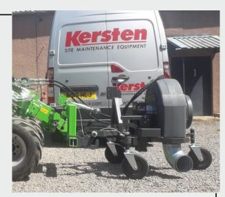
**LBV-HUT-HD/E** Hydraulic or Electric 360 degree rotational outlet chute. Use from the cab with a set of double acting spool valves or a 12 volt supply which is required to operate these accessories
